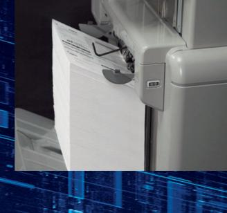
**Higher-output Capacity Finisher** New Finisher is capable to output 3500 sheets in shift printing in long runs.
